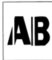
(F) White belts or streaks in the vertical direction
